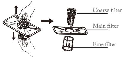
The fine filter can be pulled off the bottom of the filter assembly. The coarse filter can be detached from the main filter by gently squeezing the tabs at the top and pulling it away.
