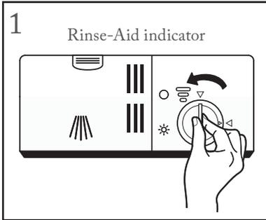
Remove the rinse aid reservoir cap by rotating it counterclockwise.
