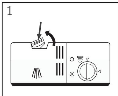
Press the release catch on the detergent dispenser to open the cover.
