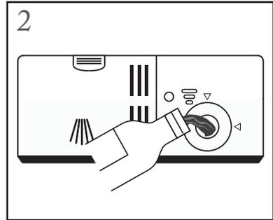
Carefully pour in the rinse-aid into its dispenser, whilst avoiding it to overflow.
