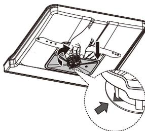
Reassemble the filters in the reverse order of the disassembly, replace the filter insert, and rotate clockwise to the close arrow.
