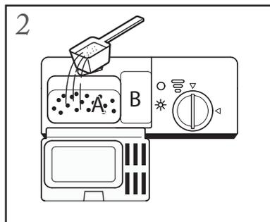
Add detergent into the larger cavity (A) for the main wash cycle. For more heavily soiled wash loads, also add some detergent into the smaller cavity (B) for the pre-wash cycle.
