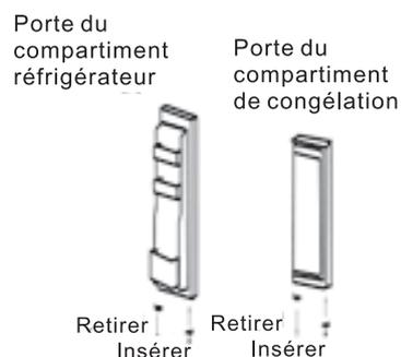
6. Place the fridge door on the lower hinge, making sure that the hinge pin is inserted in the hole at the bottom of the fridge door. Put the middle hinge back on the cabinet, making sure that it is on the opposite side from its original position.
