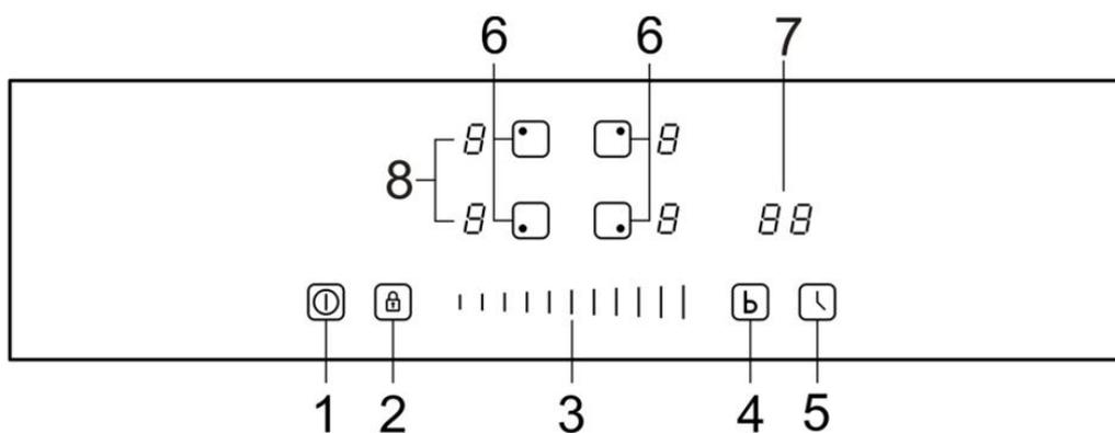
1.ON/OFF 2.Child lock 3.Select power level 4.Boost control 5.Setting the timer
