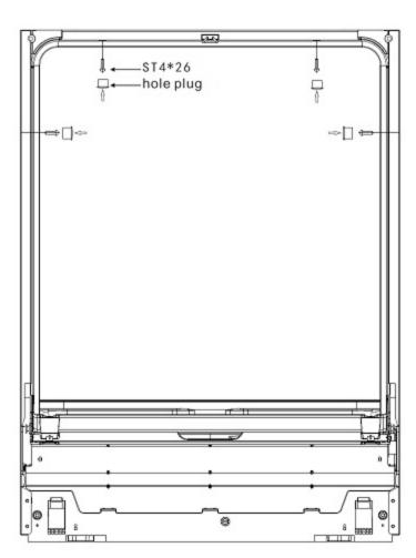
Dishwasher liner right and left side and the top 4 holes, use wood screws ST4\*26 dishwasher fixed on the cabinet (selt-tapping screws were matching)
