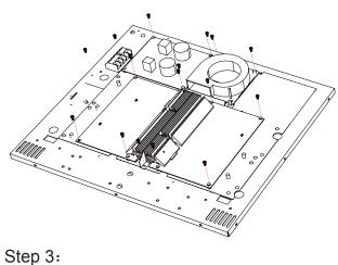
remove all the screws and wires
