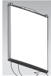
replace the door bearing bush and the limit block
