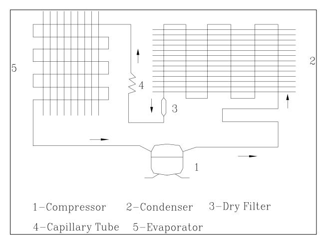
The refrigeration system of direct cooling single-system cooler belongs to the category of a single-temperature and single-control refrigerating system with one evaporators and is controlled by a single temperature control.
