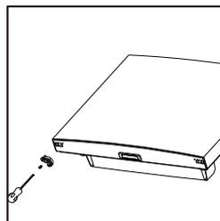
11. Install the upper door with the upper hinge.
