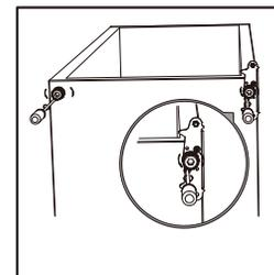
7. Unscrew and remove the bottom hinge pin, turn the bracket over and replace it.
