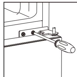
6. Laying down the refrigerator, take out the adjusting feet as below, then unscrew the lower hinge by cross screwdriver.
