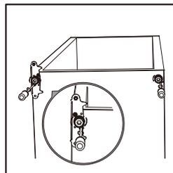
9. Make the middle hinge reverse the direction 180°, then transfer it to the left property position. Make the middle hinge pin in the upper hole of the lower door, then tight the screws.
