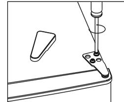
3. Remove the hole cover with a fat screw driver.
