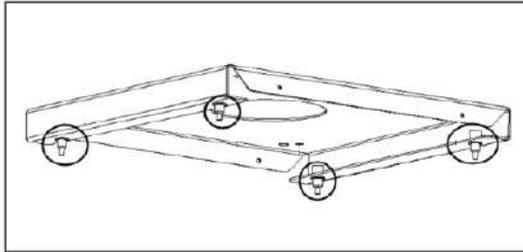
7. Position the hanging plate to the ceiling, mark the position of the holes before drilling.
