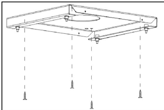
8. Assemble the decorative plant with the hanging plate with screws
