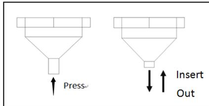
10. Lift the hood (At least two persons), and connect the hood with the hanging plate using 4 cables. Insert the cables to the cable holders which on the cooker hood. Adjust the cable length.
