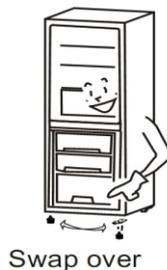
5. Remove the hinge pin that is in the bottom of the fridge and freezer door. At the other side of the fridge and freezer door, insert the replacement hinge pin that is supplied with the appliance.
