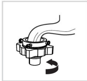
Tighten clamp nut
