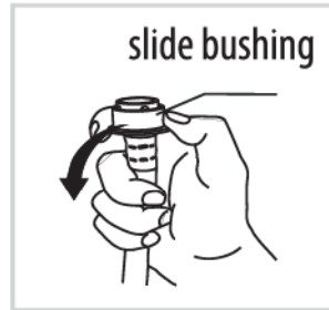
Press slide bushing, insert inlet hose into connecting base
