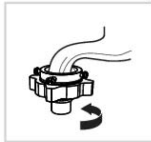
Tighten clamp nut
