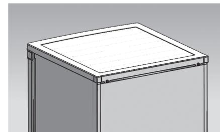
2. Remove the top-hinge fixing screws with cross-slot screwdriver. Take off the door and put it down with care in a safe location.
