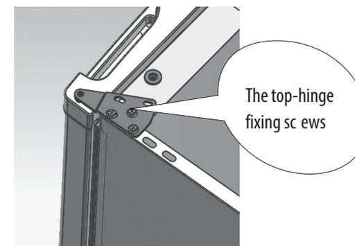
The top-hinge fixing screws
