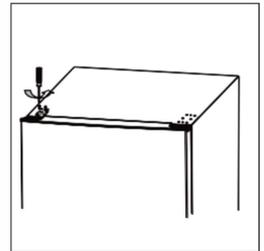
13. Fix the hinge cover on the left and the hinge hole cover on the right
