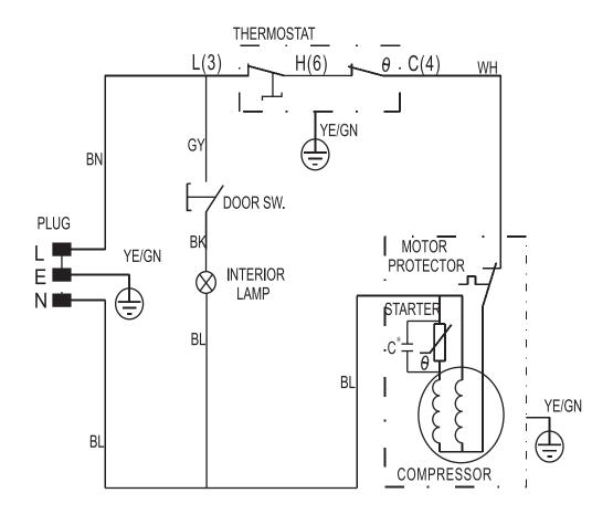
C\*: The capacitor is optional according to different compressor model
