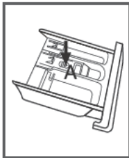
Pull out the dispenser drawer with press the A
